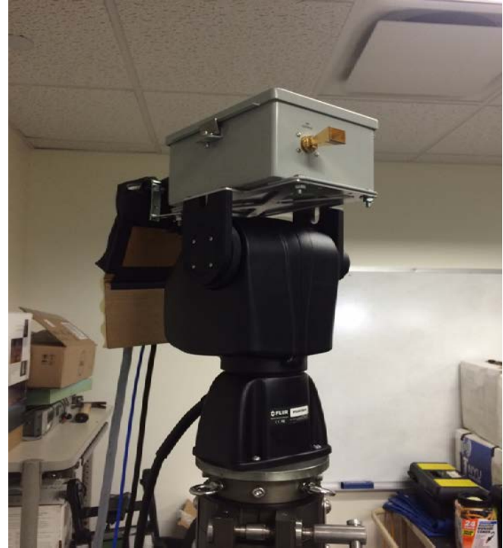
*Note: 20 dBi horn antenna on upconverter
